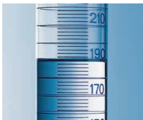
BLAUBRAND®. Ring marks at major graduations. Reading at lowest point of meniscus.
